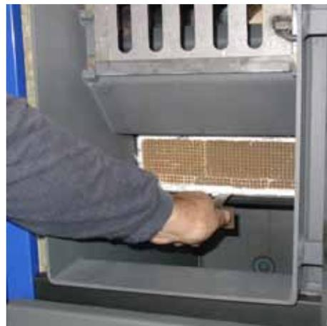
Easy to handle! The catalytic converter in its box
